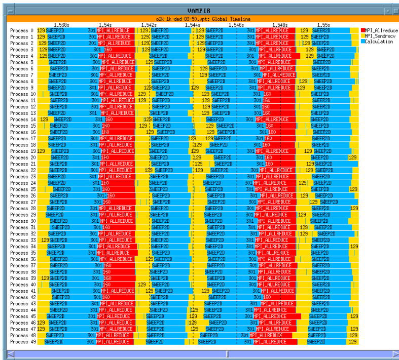
Figure 30: One of the Jacobi iterations (NX=1000), running on 50 processors of a dedicated Origin2000
