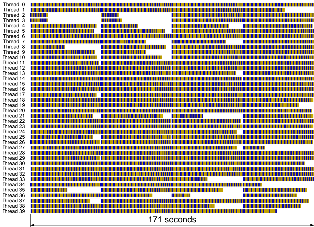
Figure 33: Runtime behavior of a multi-threaded kernel with maximum data access collision
